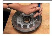
1. Follow the factory service manual to remove the clutch basket from the motorcycle. Once the clutch basket has been removed from the bike remove the clutch plates from the basket. It is not necessary to remove the drive hub for this procedure. Use a center punch to mark the center of the rivets to be drilled out and removed.
