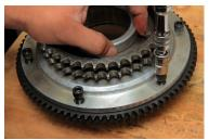
5. Use Red thread lock on the provided mounting bolts ( $5/16''-24 \times 5/8''$ ) and torque to 15-18 Ft/lbs. Then re-install the clutch components and any remaining items per the factory service manual. It is recommended to replace the starter motor pinion gear at the same time as replacing the ring gear.
