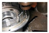
3. Ream all of the clutch basket rivet holes with a 21/64" drill bit. Clean up all loose material or burrs from the holes. Check to see that the holes are big enough to fit the new ring gear bolts provided in the kit.
