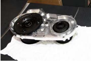
View after front pulley is installed to motor plate.
